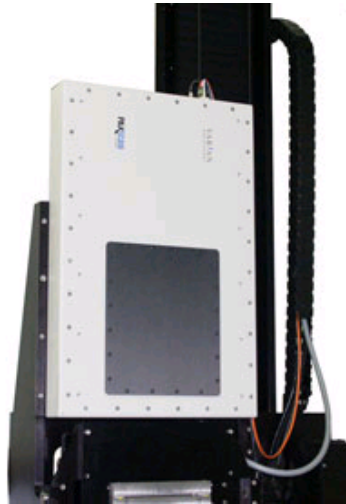
Flat panel detector with shielded electronic components
